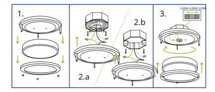
Step1: Unscrew three cap nuts counter-clockwise, remove metal ring and the lens.
