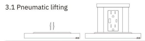
Press the top glass surface to lift / lower the socket.
